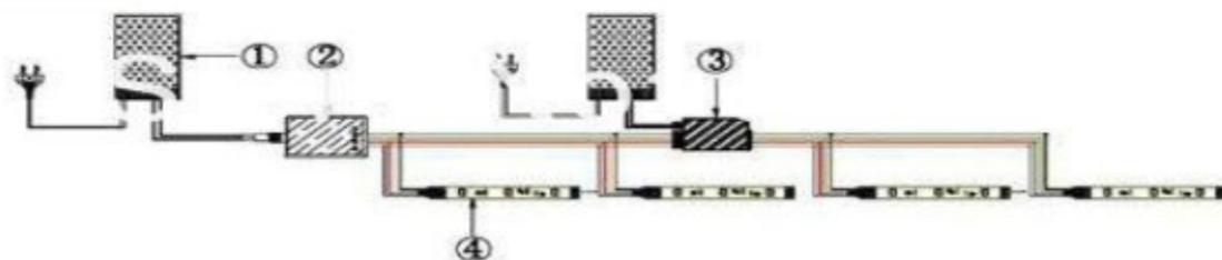
① Power Supply ② Controller ③ Amplifier ④ LED Strip
