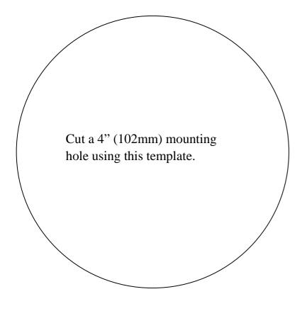
Place the water-proof ring with O-ring on the mounting hole first. Fasten the clear lid / conversion solar kit to the water-proof ring using 3 s.s. wood screws (M4 x 43mm length) as fig. 1.
